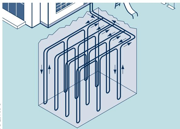
**A typical GHP system, such as this elementary school application, circulates water through ground-source heat exchangers to provide space heating/cooling and hot water.**
