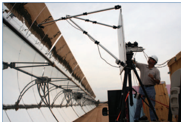
NREL's VSHOT laser scanning system determines the accuracy of concentrator mirror structures and is used in both a laboratory setting and in the field. It has proven critical in the design of new reflector structures.
