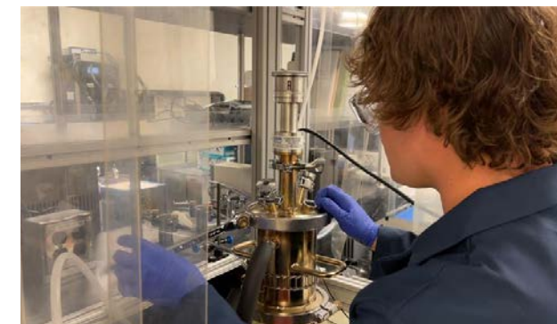
A researcher uses a 1-L reactor in NREL’s energy storage laboratory to evaluate black mass from recycled battery electrodes.
