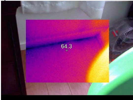
Air leakage from vented crawl space
