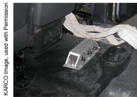
Figure 3. Mounting of the sensor bracket and sensors in the test vehicle
