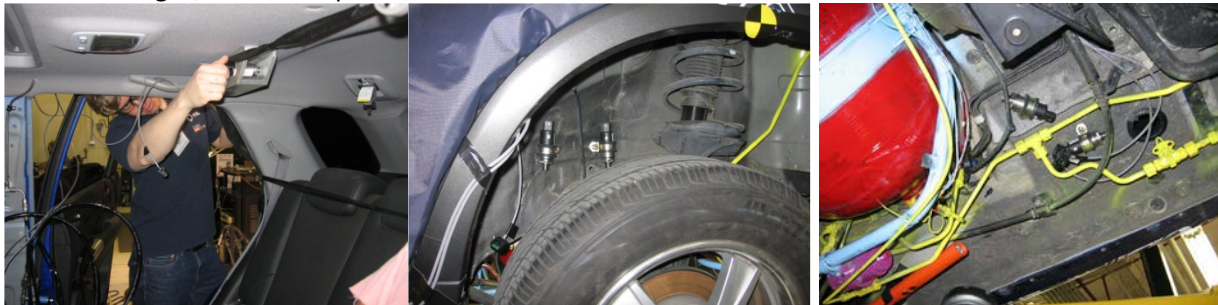
Figure 5. Mounting of the sensors in a FCEV
