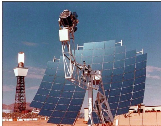
Figure 3. Parabolic (near) and tower (background) solar concentrators
