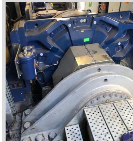
Instrumented gearbox in the SGR G97 turbine. Photo by Jerry Hur, NREL
