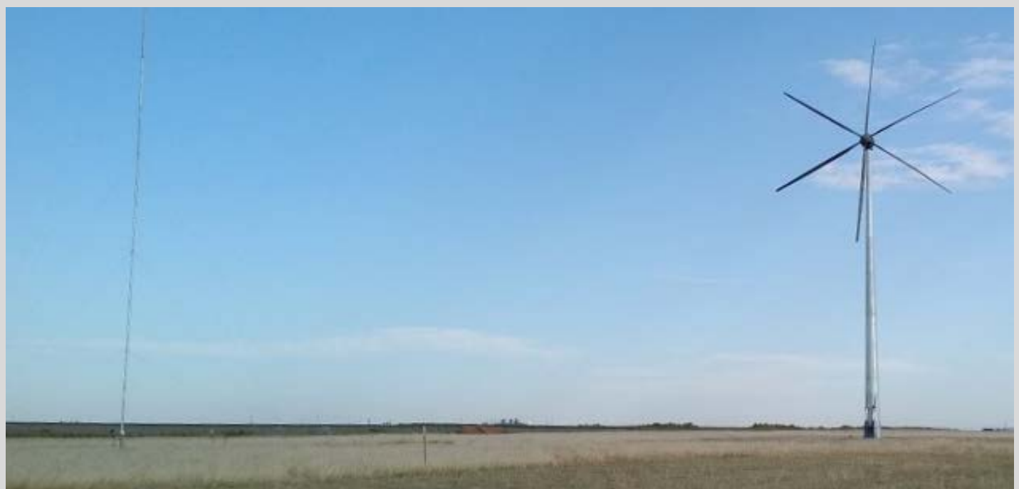
Star Wind Turbines in East Dorset, Vermont, is in the process of testing and certifying their six-bladed Star72 turbine (like this one on a monopole tower at the RenewTest facility in Pampa, Texas) to the new American Clean Power 101-1 standard. Photo from David Carr, RenewTest
