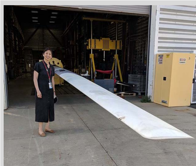
Lucy Pao, a joint appointee at CU Boulder and NREL, stands next to a segmented ultralight morphing rotor wind turbine blade at NREL's Flatirons Campus shortly after the blade was manufactured and delivered to the lab for DOE-funded experiments in July 2018. The ultralight, flexible wind turbine rotor, designed by a multi-institutional team that included Pao and other NREL researchers, could lower wind energy costs. Photo by Kathryn Johnson, Colorado School of Mines/NREL
