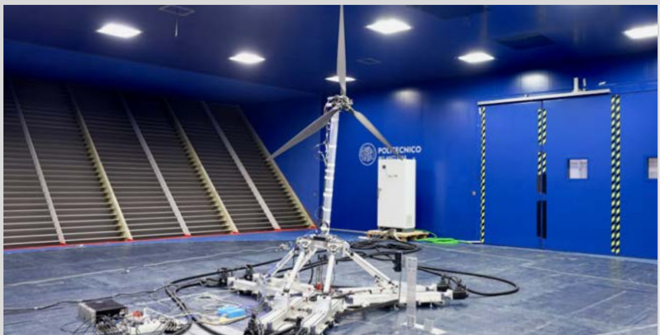
Experiments are conducted on a scaled version of a 10-MW reference wind turbine in Politecnico di Milano's wind tunnel using a robotic system to mimic the motion of the wind turbine in the open ocean. This research provides a better understanding of how to model the aerodynamics of floating wind energy systems, enabling the development of more reliable and optimized designs. Photo from Alessandro Fontanella, Politecnico di Milano
