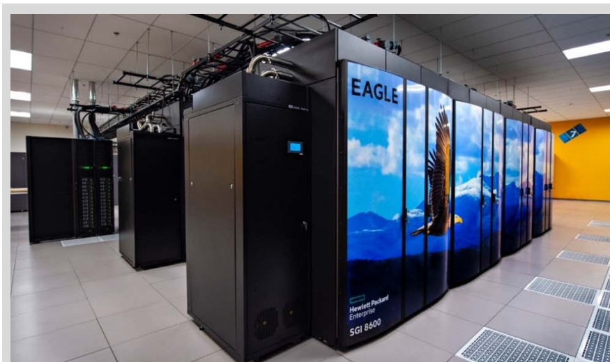
NREL's high-performance computing data center houses Eagle, an 8-petaflop supercomputer. Photo by Dennis Schroeder, NREL
