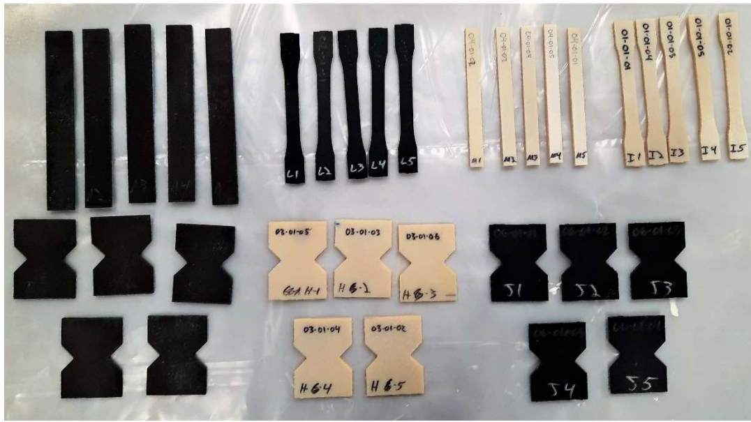
Figure 2. A photo of some of the test specimens that were prepared for environmental conditioning (photo by Paul Murdy, NREL).
