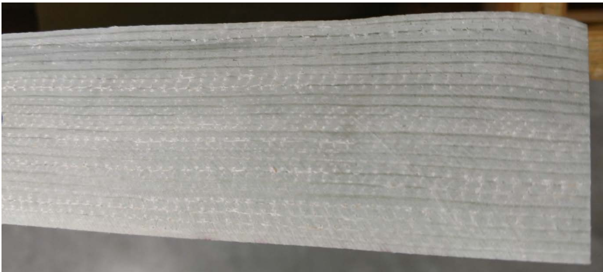
Figure 2. Cross-sectional view of a manufactured thick panel
