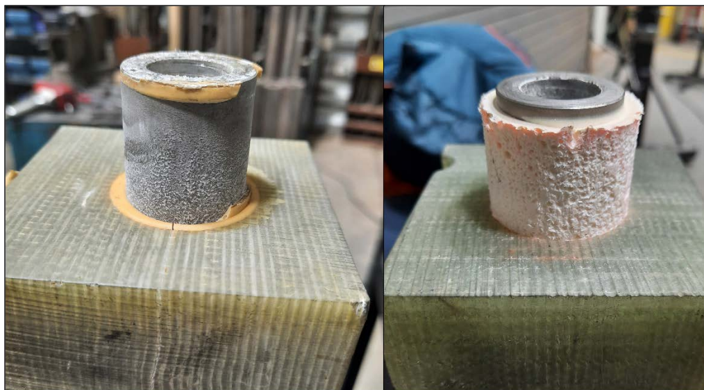
Figure 47. Photographs demonstrating the differences in failure modes observed between the (left) Araldite and (right) Plexus DEI specimens
