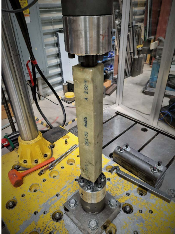
Figure 22. A DEI specimen set up in the load frame prior to testing to failure
