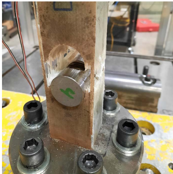
Figure 42. A typical through-hole tensile failure observed for all the T-bolt specimens tested under fatigue loading
