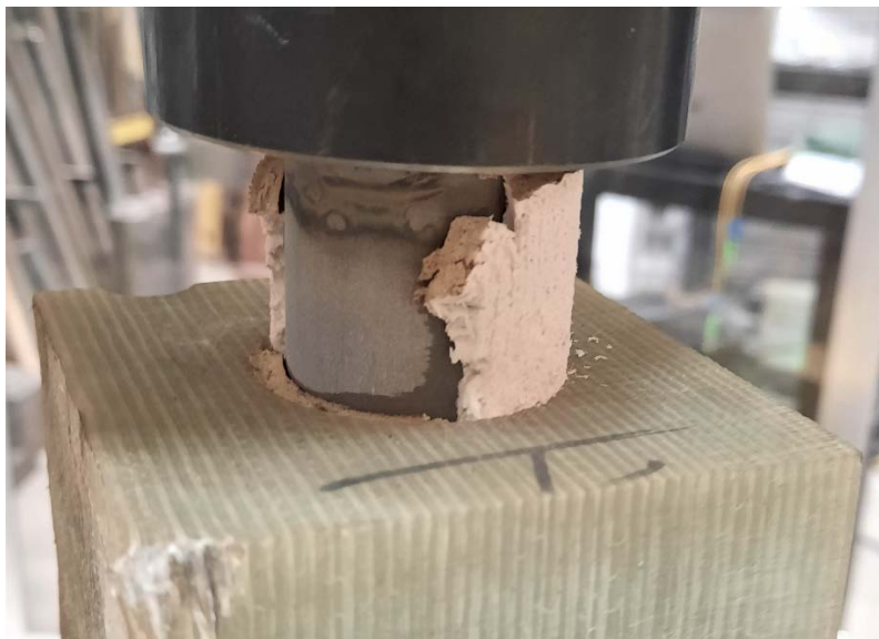
Figure 45. Moisture observed deep in the adhesive bondline of a DEI specimen with Plexus adhesive
