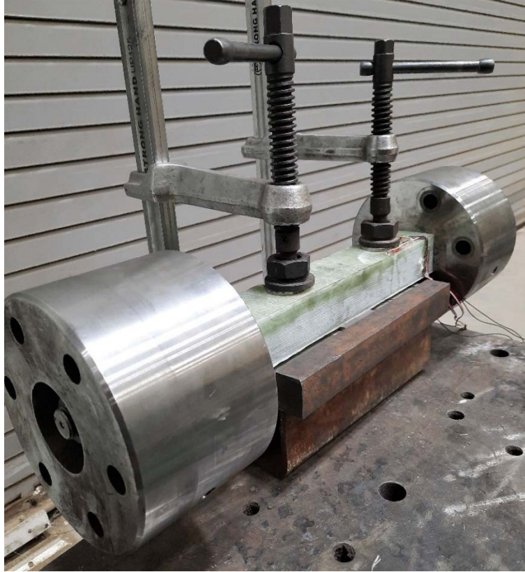
Figure 20. A T-bolt specimen being loaded into the test fixture using the alignment fixture
