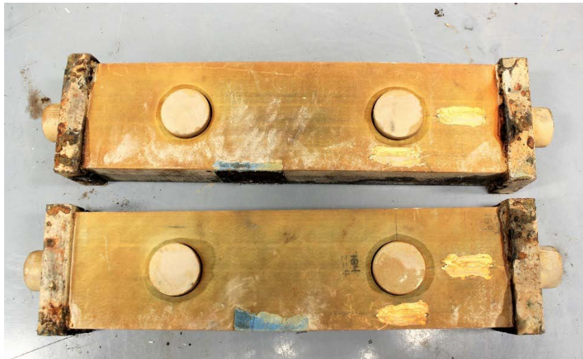
Figure 29. Extensive amounts of corrosion (iron oxide) stuck to the surface of T-bolt specimens with broken fiber optic gauges attached
