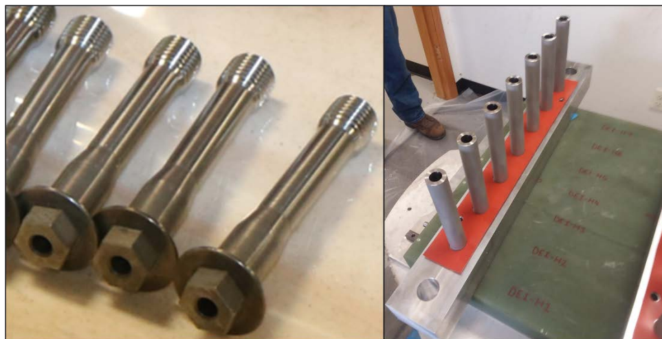
Figure 10. (left) An M20 injection bolt used to inject adhesive into the cavity between the inserts and the composite blank and (right) a photo of the inserts bolted to the end bars in preparation for bonding
