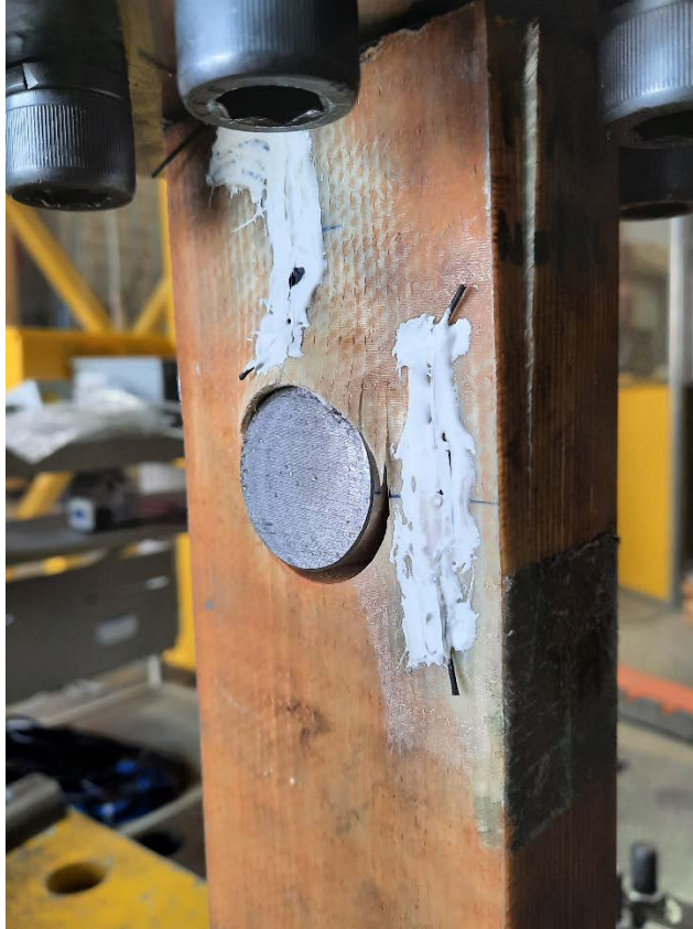
Figure 38. An example of a through-hole bearing failure exhibited by all the T-bolt specimens tested under static loading conditions
