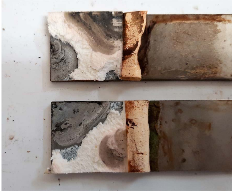
Figure 51. Corrosion observed deep in the bondlines of 316 steel MMLS specimens conditioned at PNNL
