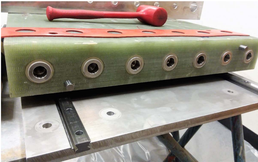
Figure 11. A composite blank with the adhesive bonding process complete
