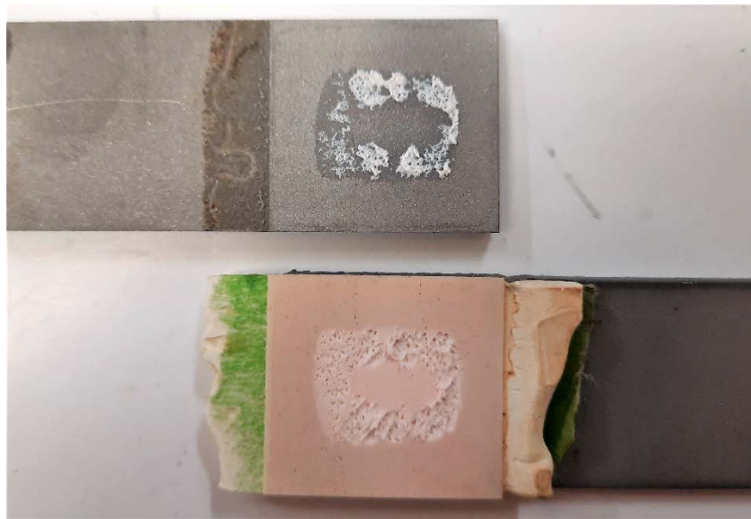
Figure 52. Mixed adhesive/cohesive failure of a Plexus MMLS specimen conditioned at FAU
