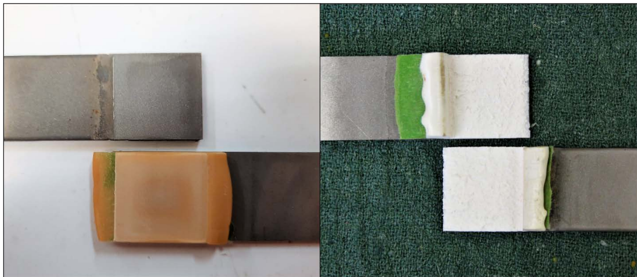
Figure 50. A comparison of failure modes observed in the (left) Araldite and (right) Plexus MMLS specimens
