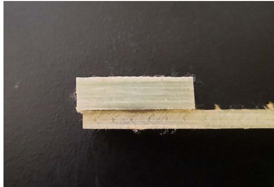
Figure 24. A fiberglass end tab bonded to a CCLS specimen to ensure good alignment in the load frame
