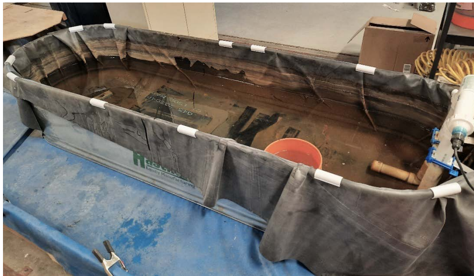
Figure 18. Cold-water storage tank used to maintain saturation conditions of specimens prior to mechanical testing
