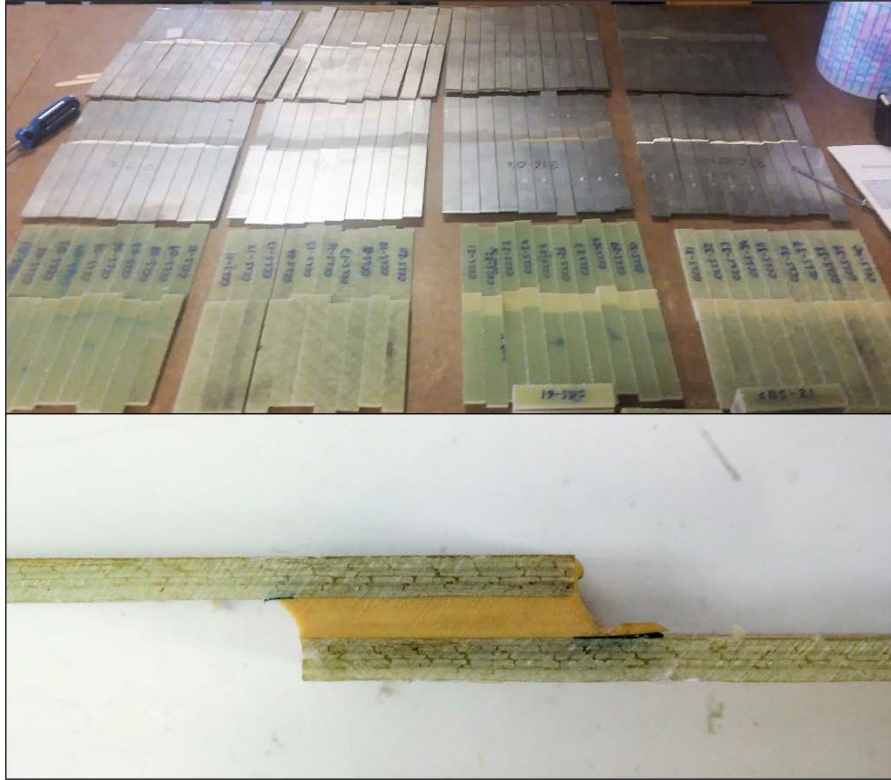
Figure 15. (top) The final manufactured MMLS and CCLS specimens and (bottom) a closer view of a CCLS bondline cross section
