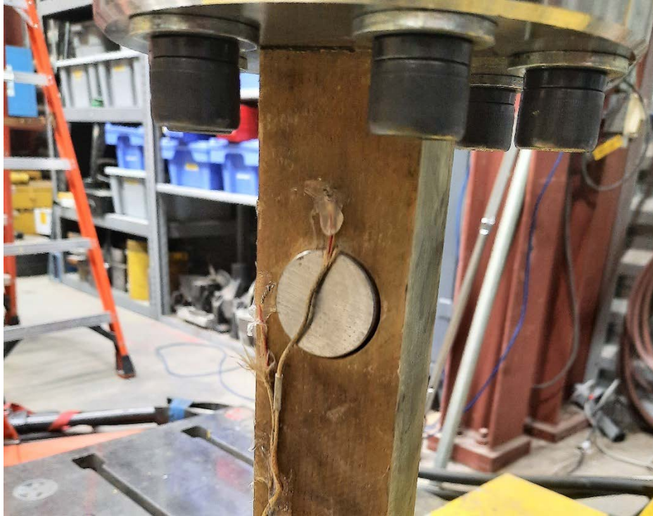
Figure 21. Thermocouples bonded to a T-bolt specimen for fatigue testing
