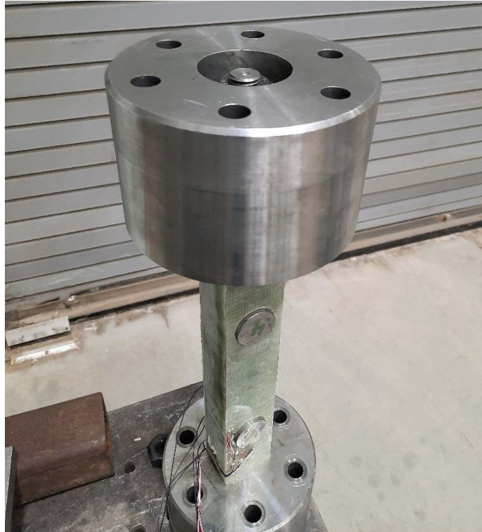
Figure 19. The fixture used to connect the T-bolt specimens to the 500-kN load frame
