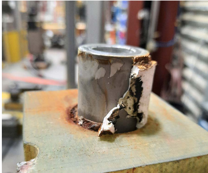
Figure 46. Corrosion observed in the adhesive bondline of a DEI specimen with 316 steel inserts that was conditioned at PNNL
