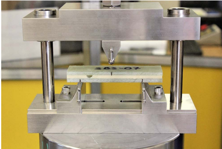
Figure 26. An SBS specimen prepared in the three-point bend fixture before loading to failure
