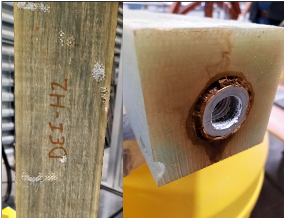
Figure 32. (left) Discoloration and streaking on the surface of a Hexion DEI specimen conditioned at FAU and (right) corrosion observed on a 316 steel insert of a DEI specimen conditioned at PNNL
