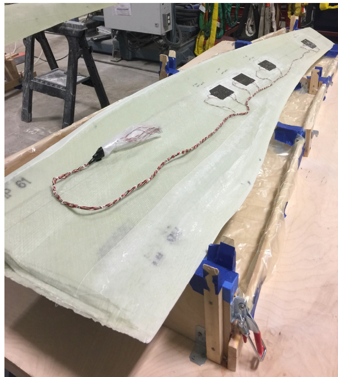
Figure 4. Blade 2 high-pressure skin with strain gage instrumentation for Channels 8–10 (given in Table 1). From left to right these are named SG07-BL2-1100-FB-SC, SG08-BL2-1300-FB-SC, SG09-BL2-1575-FB-SC, and SG10-BL2-2200-FB-SC.
