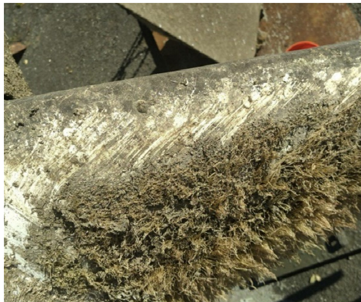
Figure 12. Marine growth on blade.
