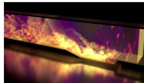
Direct fuel injection in supersonic cavity flame-holder 1 .
