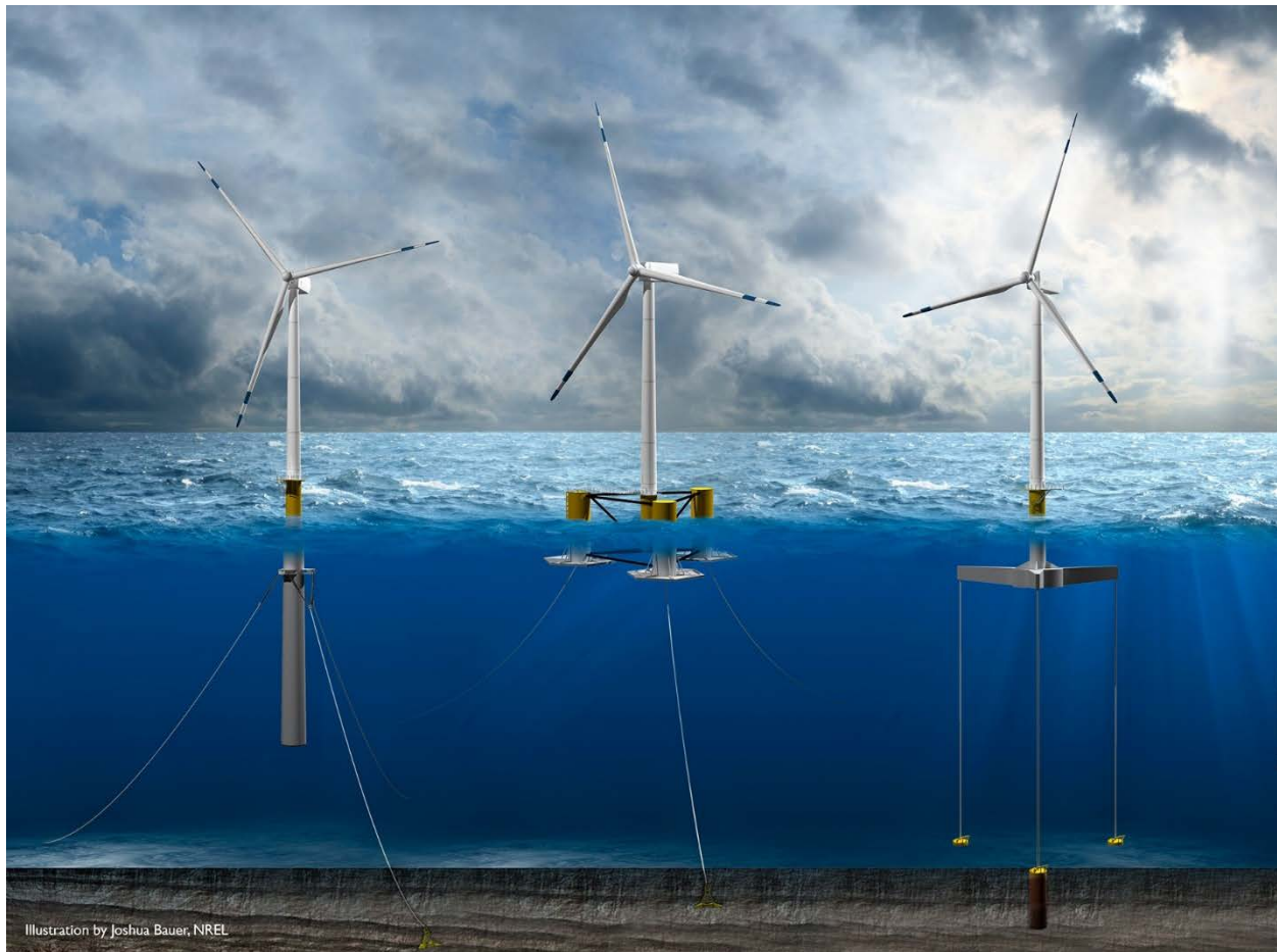
Figure 3. Examples of floating substructure types: spar (left), semisubmersible (center), and tension-leg platform (right). Illustration by Joshua Bauer, NREL
