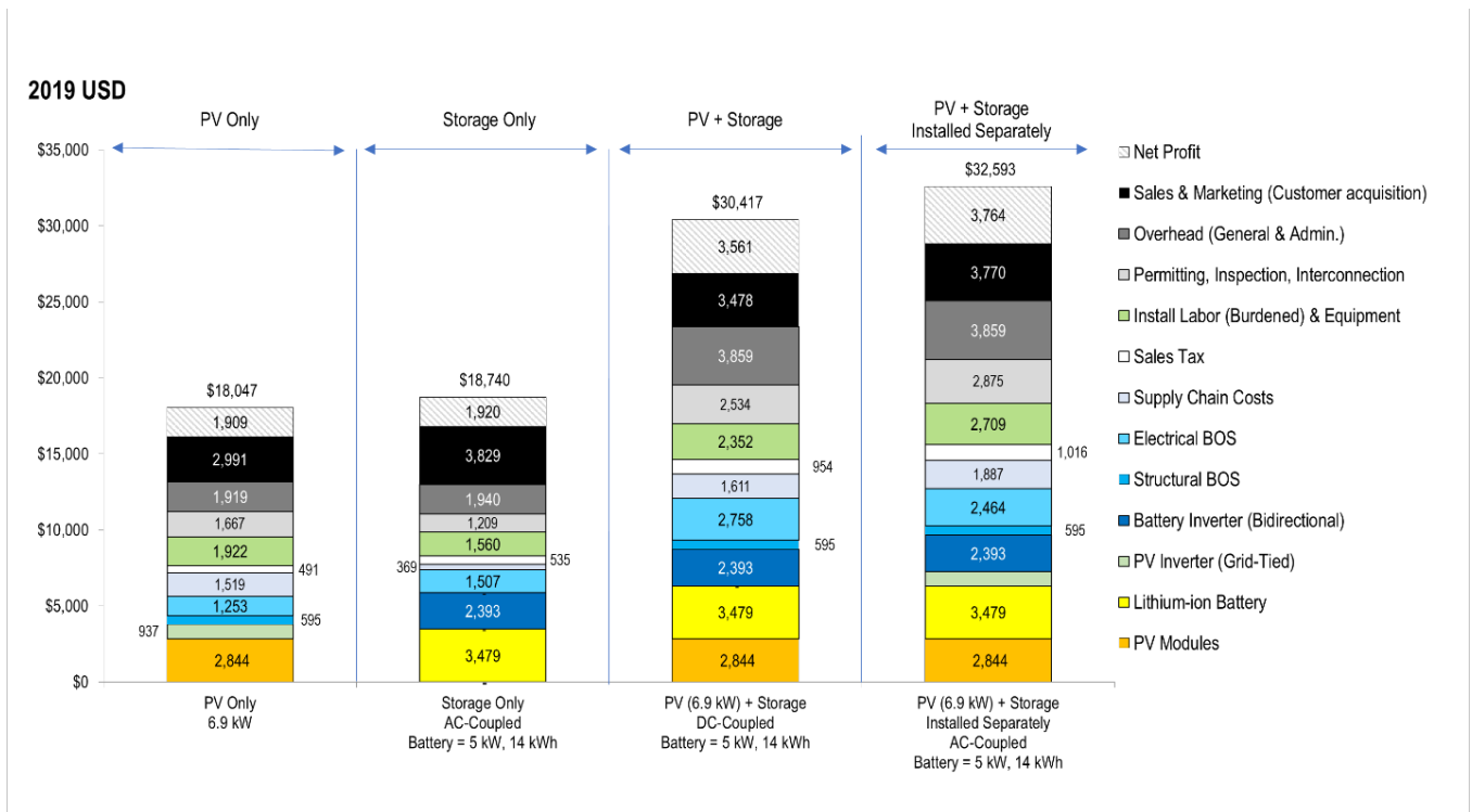
Figure 2. Cost of residential PV stand-alone, battery storage stand-alone, and PV + battery storage systems estimated using NREL bottom-up models (Augustine and Blair 2021)
