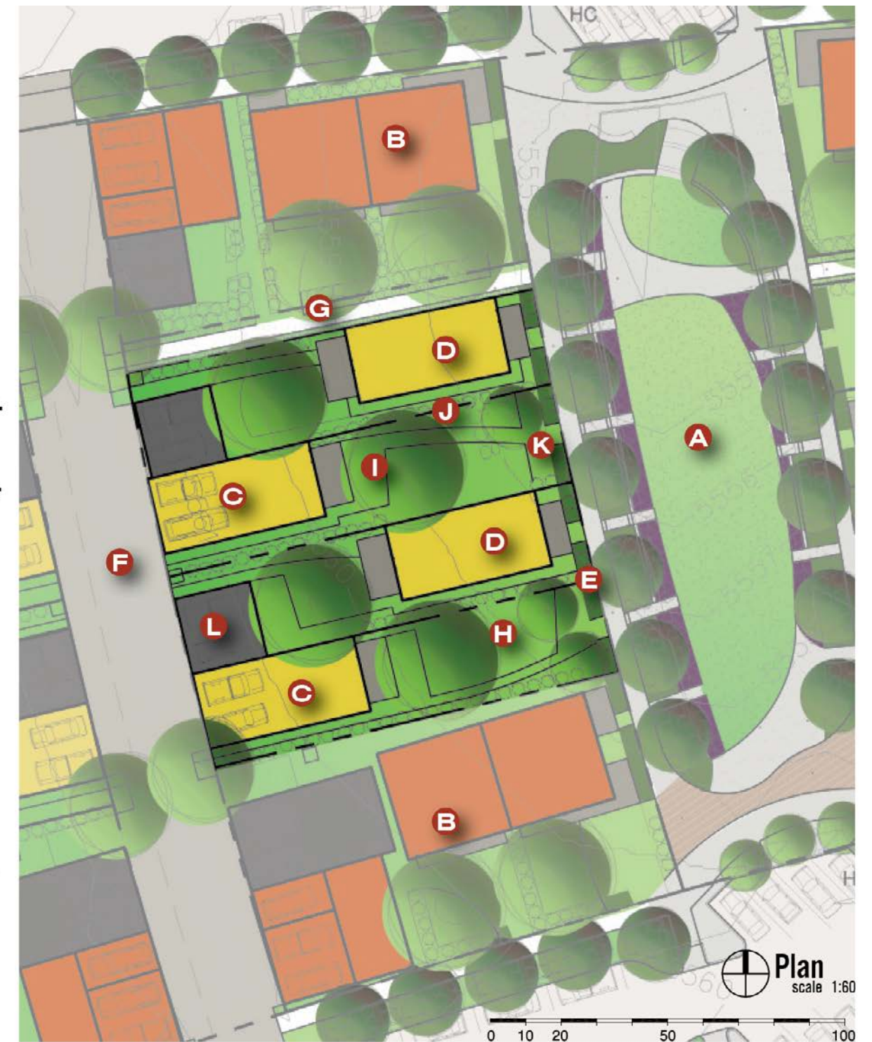
FIGURE 40. The Geos Neighborhood master plan ensures solar access for all buildings with a checkerboard pattern of homes and landscaping
