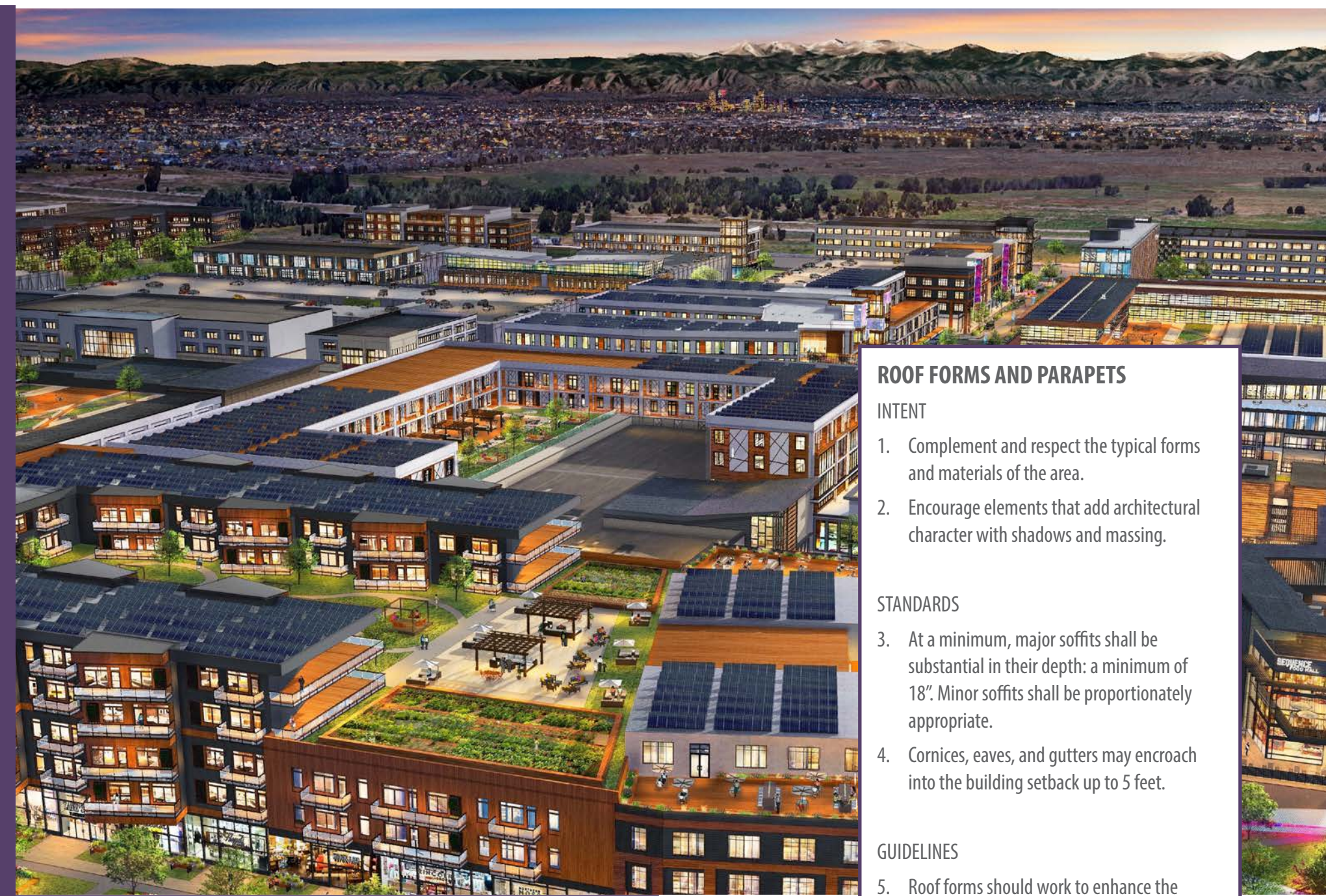
FIGURE 42. Guidance on using roof forms and parapets to optimize the roof areas available for solar photovoltaics from the Peña Station NEXT design standards
