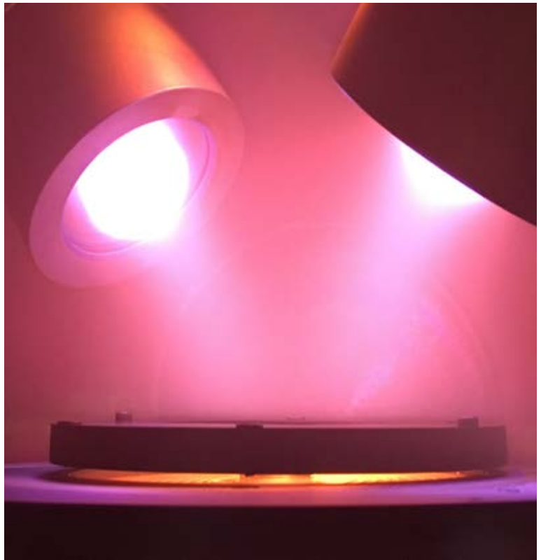
Thin-film growth in reactive plasmas. Photo by Andriy Zakutayev, NREL
