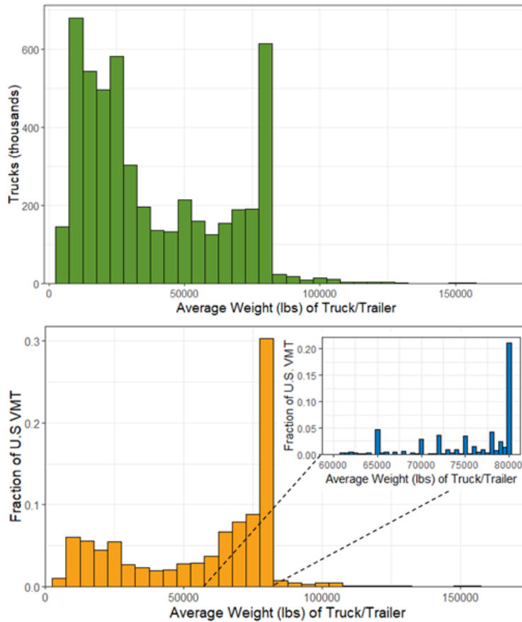
Figure 9. VIUS data on average weight of a truck/trailer by (top) count and (bottom) VMT fraction when they are operated with a typical payload over the year
