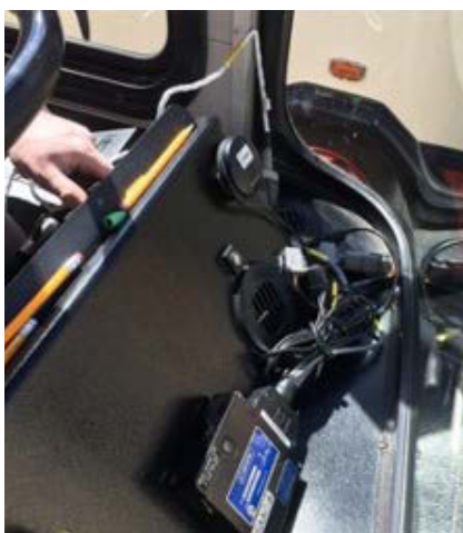
Figure 2. Example of a data logger placed on a bus. Photo credit: NREL
