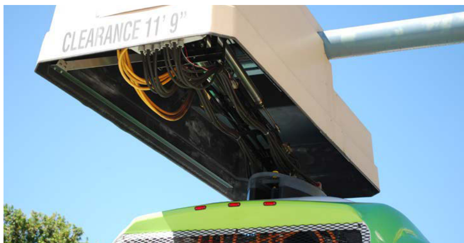
Figure 1. Proterra fast-charge electric bus charging station photo by: Leslie Eudy, NREL
