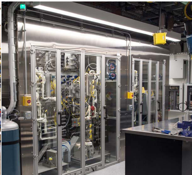
The Fuel Synthesis Catalysis Laboratory is a newly renovated 1,120-square-foot laboratory space that houses six semi-automated reactor systems with online gas chromatography product analysis. Photo by Dennis Schroeder, NREL 51117
