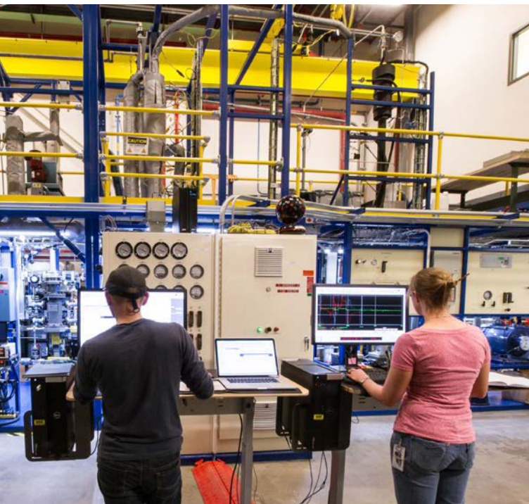
NREL engineers evaluate bio-oil co-processing using the 2,000-square-foot Davison Circulating Riser Reactor Laboratory.
