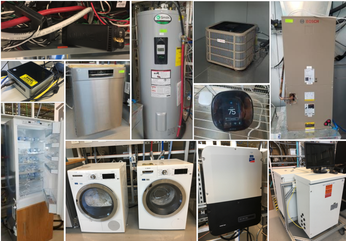
Figure 15. Appliances used in the laboratory experiments. Clockwise from top left: Neurio power meter (Wi-Fi), AO Smith electric water heater (CTA-2045), Bosch air-source heat pump, ecobee4 thermostat (ecobee cloud API), Eguana home battery (Modbus), SMA SunnyBoy inverter (SunSpec), Bosch clothes washer and dryer (HomeConnect cloud API), Bosch refrigerator (HomeConnect cloud API), Intel NUC minicomputer running foresee, and Bosch dishwasher (HomeConnect cloud API).
