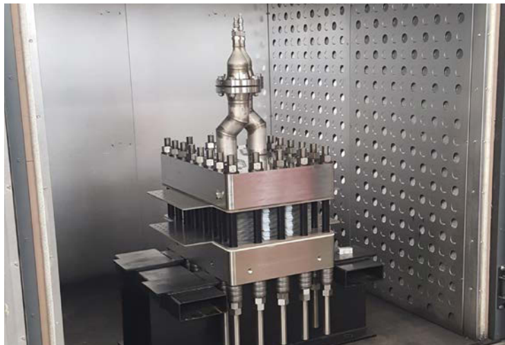
Giner ELX's high-current-density, megawatt-scale electrolyzer stack. Engineers at the ESIF will validate the efficiency and durability of the new stack design. (Photo by Monjid Hamdan/Giner ELX)
