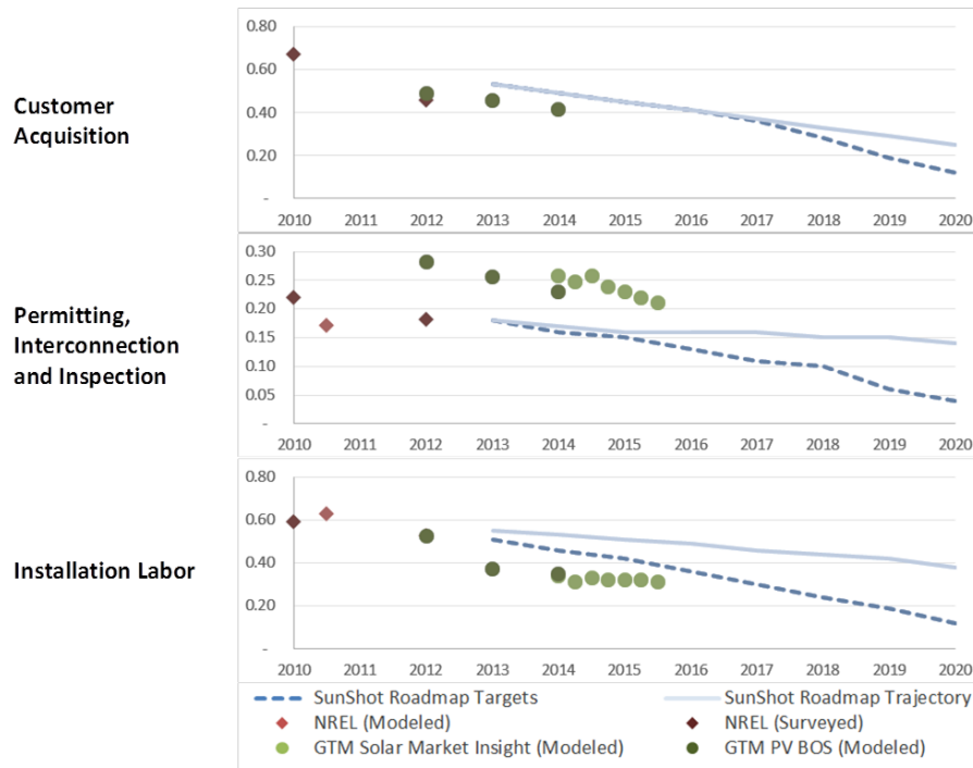
Figure 4. Summary of recent values for residential solar soft costs (2010$ per watt DC)
