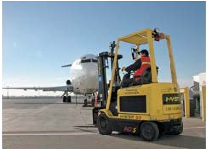
Figure 3. A hydrogen fuel cell forklift in airport service. Photo courtesy of Hydrogenics, NREL 15987
