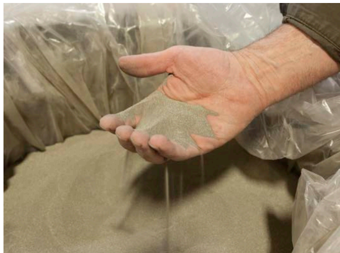
NREL developed, patented, and licensed this catalyst, which removes tars to makes thermochemically derived biomass syngas ready for fuel synthesis.
