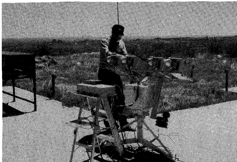
Figure 3-5. Outdoor intercomparison of four spectroradiometers
