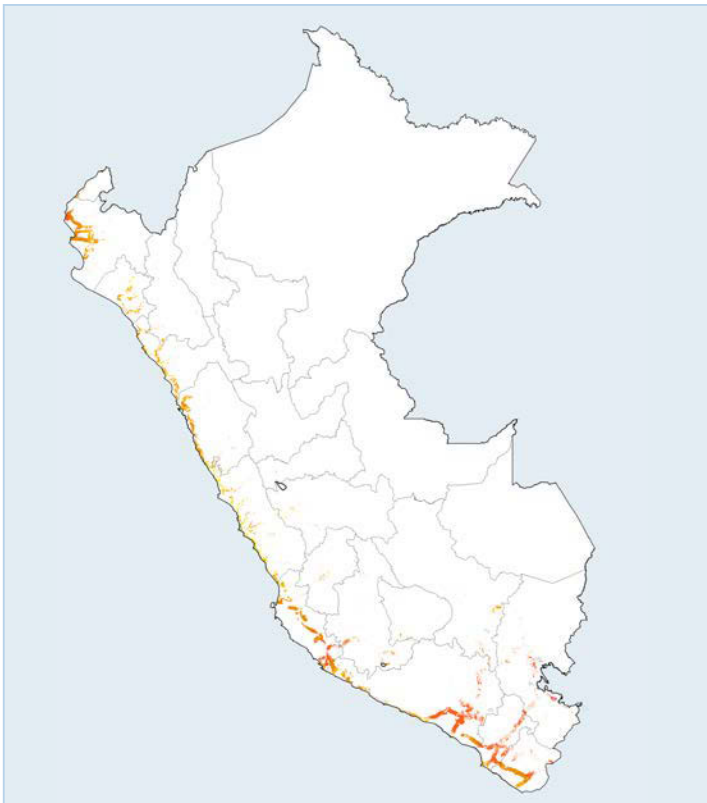
Figure 3. RE Data Explorer results for PV technical potential – each dot represents a 4 km x 4 km square that meets analysis constraints. Color corresponds to GHI bin.
