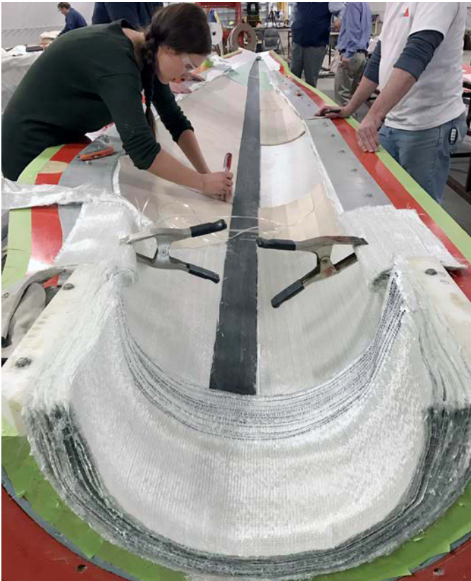
The team works to develop a blade using recyclable thermoplastic materials. Photo by David Snowberg, NREL 41767
