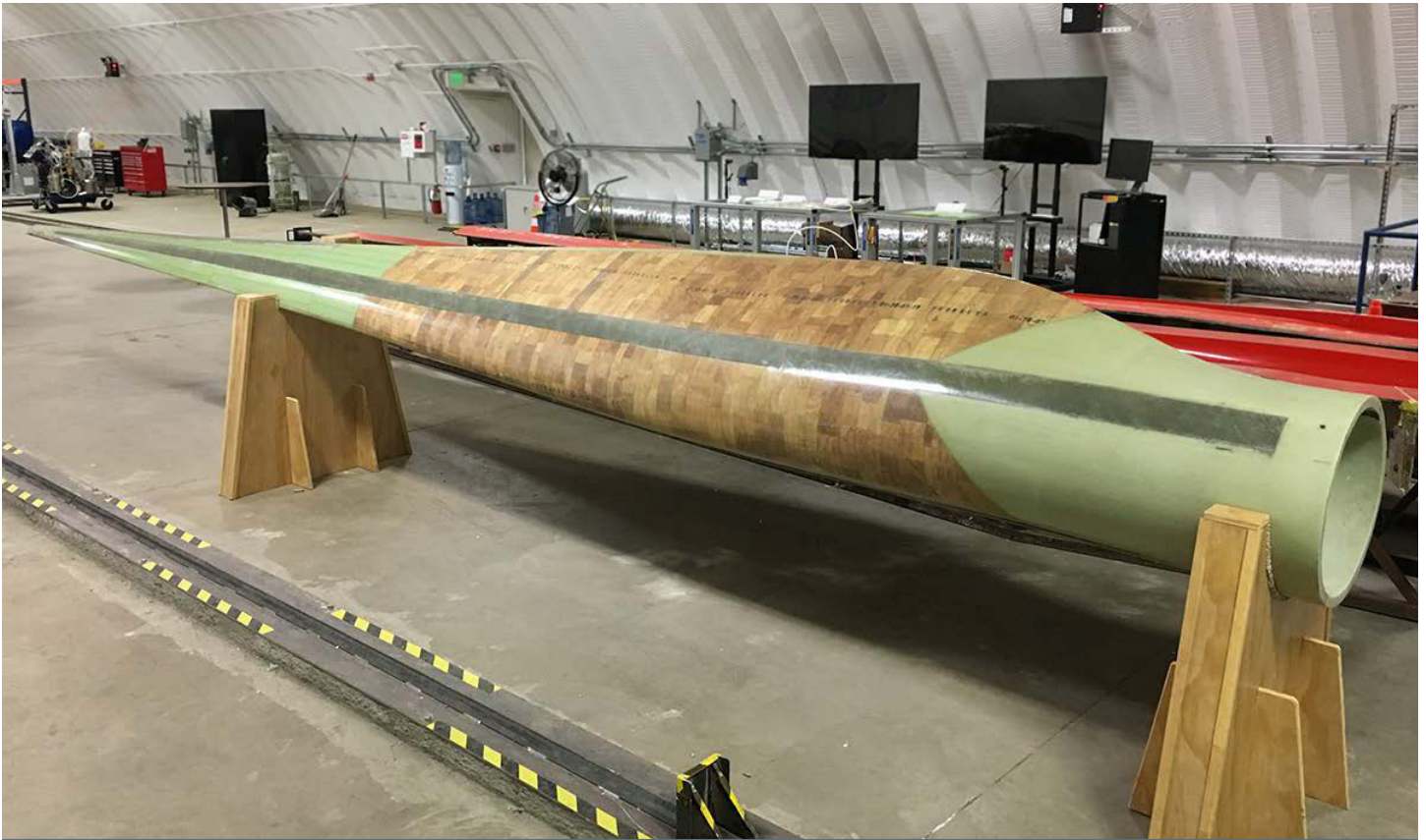
NREL researchers used advanced composite materials to create a 9-meter recyclable thermoplastic wind turbine blade. Photo by Samantha Rooney, NREL
