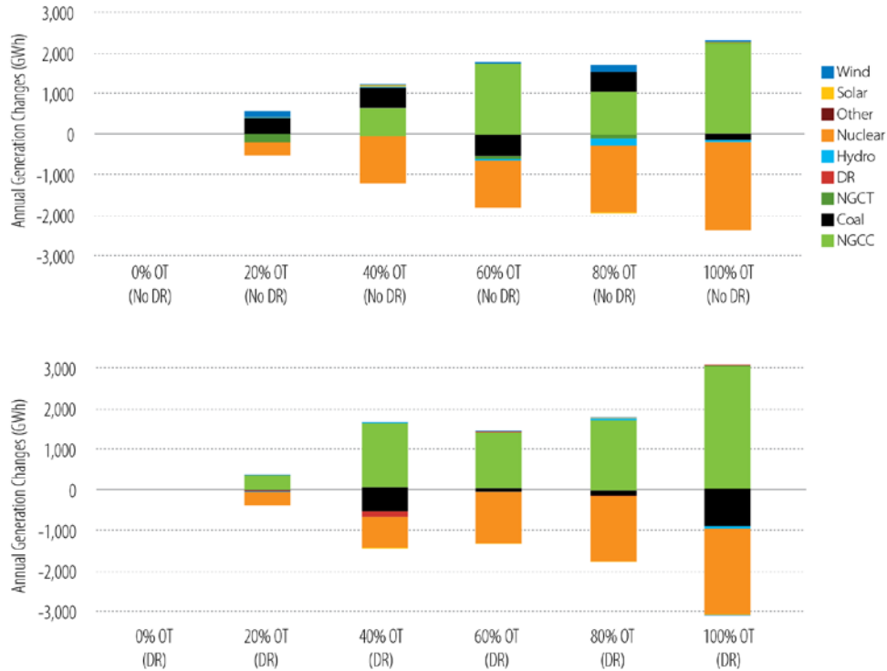
Figure ES - 2. Total annual generation differences for scenarios with thermal curtailments minus scenarios without thermal curtailments in cases without DR (top) and with DR (bottom)
