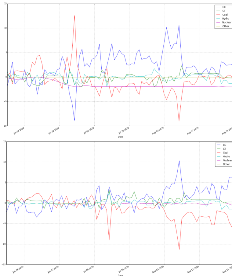
Figure D - 1. Comparison of generation mixes on an hourly basis for summer months (June, July, and August) for 100% recirculating cooling thermal systems (top) and 100% once-through cooling systems (bottom) with no curtailments compared with the baseline scenario
