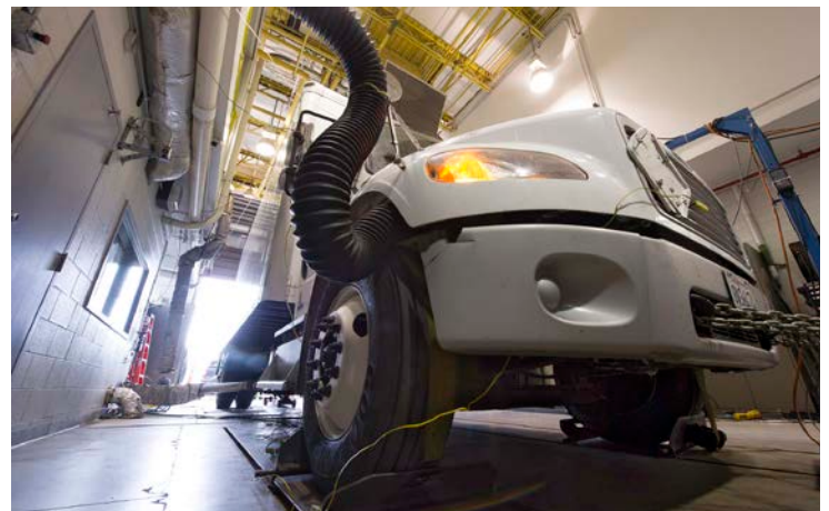
A fleet vehicle being tested on the chassis dynamometer at ReFUEL Photo by Dennis Schroeder, NREL 22772
