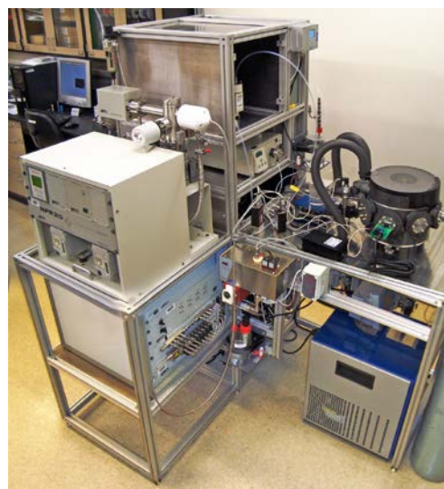
Figure 2: Hydrogen sensor testing facilities of JRC-IET (left) and NREL (right)
