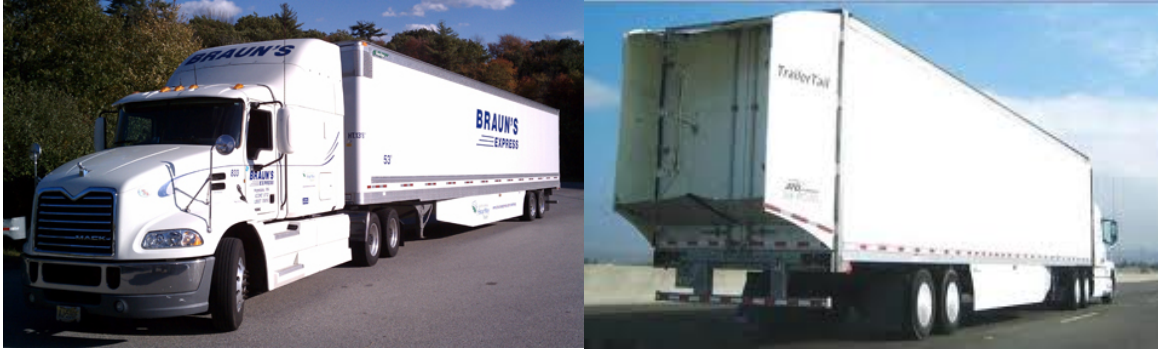
Figure 2.5. Aerodynamic devices on a tractor-trailer: side skirts and boat tail
