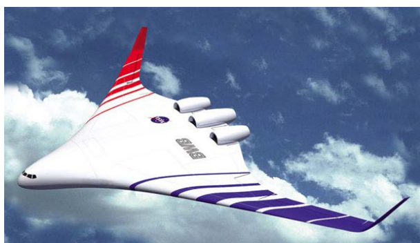
Figure 3.4. Blended wing body
