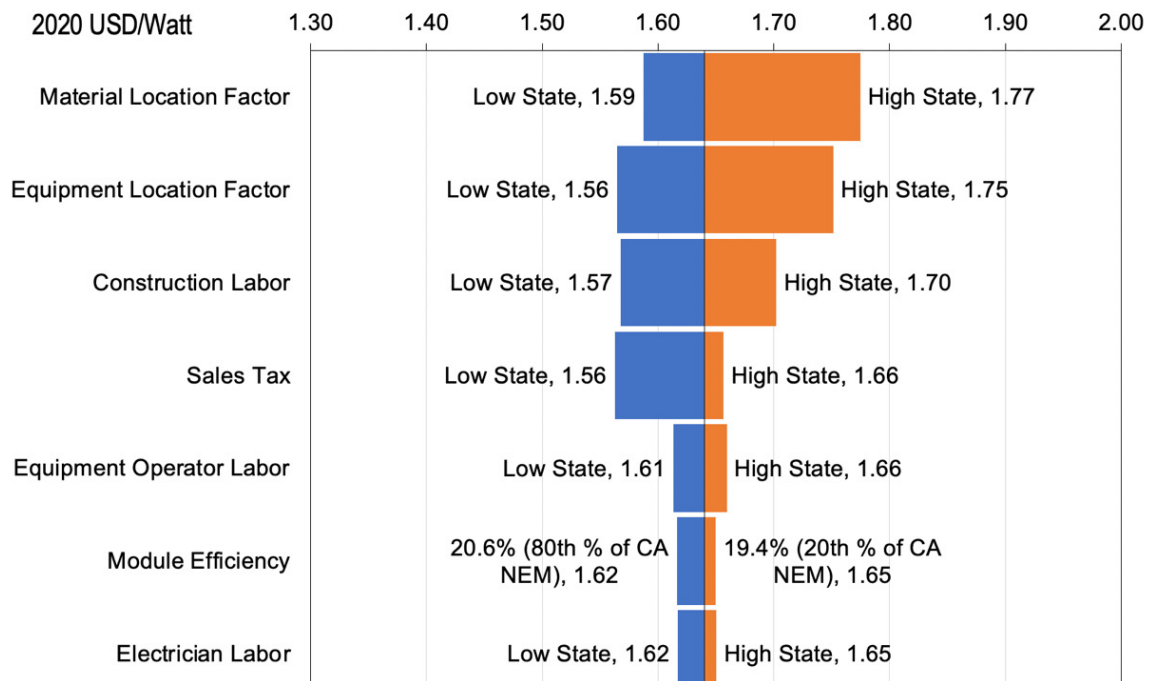
Figure 9. Sensitivity analysis for the Q1 2021 benchmark: 500-kW commercial ground-mounted PV system cost (2020 USD/W DC )
