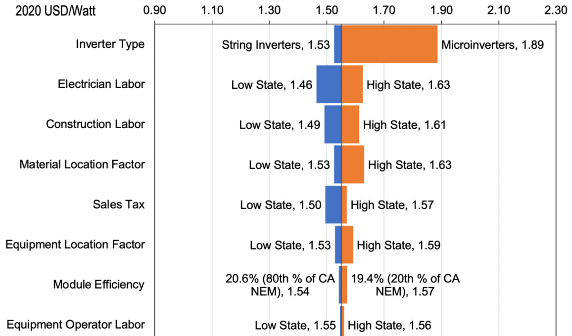
Figure 8. Sensitivity analysis for the Q1 2021 benchmark: 200-kW rooftop commercial PV system cost (2020 USD/W DC )
