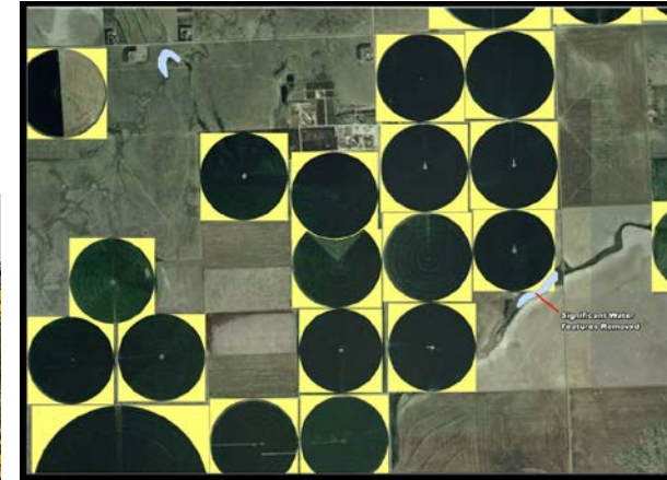
Tapping solar resources in non-irrigated corners of center pivot irrigation fields. Source: Roberts, B. NREL Technical Report. TP-6A20-51330, 2011
