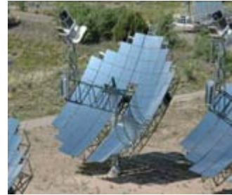
Figure 5.1.3. The Stirling Energy Systems 25-kW dish/Stirling system is undergoing operational testing at Sandia National Laboratories in Albuquerque, NM.
