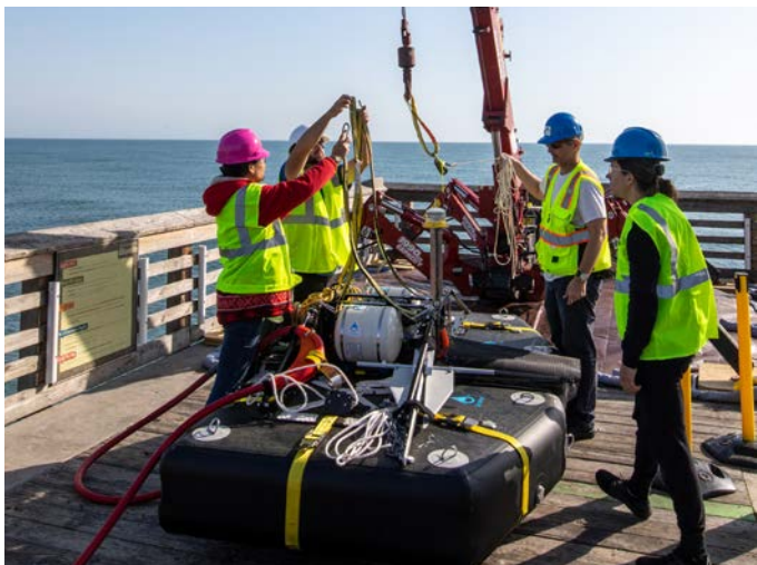
Waves to Water Prize finalists deployed and tested their wave-powered desalination prototypes in North Carolina in April 2022. Photo by Werner Slocum, NREL
