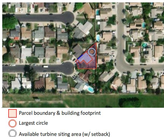
Figure 4. Satellite image of an example behind-the-meter parcel and its associated geographical boundaries located in northern California. Image from Google (2021)
