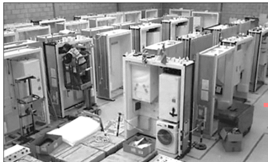
FIGURE 28 The Battersea project involved producing 540 utility cupboards for apartments in a major real estate development in the United Kingdom. Source: RIBA 2013.
