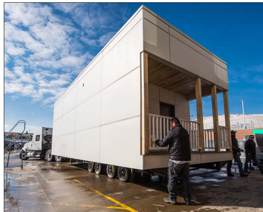
FIGURE 2 An iUnit apartment is tested at the Outdoor Research Block at NREL in Golden, CO. This research area accommodates research, development, and testing on energy efficiency in modular apartment units. Source: NREL.
