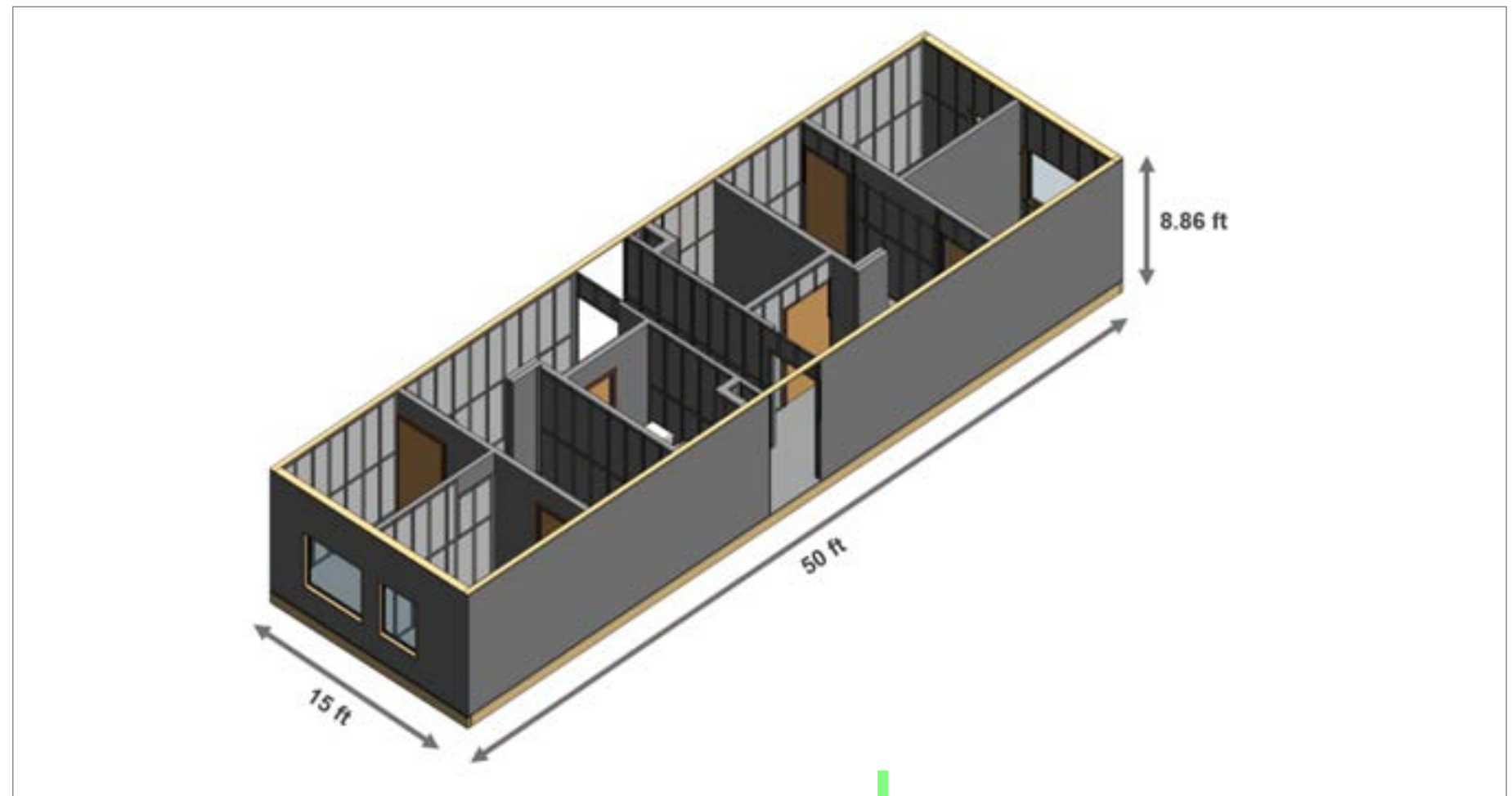
FIGURE 21 Baseline 3D model of modular unit showing wall framed with traditional 2x6 studs at 16" o.c., framed in the factory. After the modular unit gets shipped to site and stacked along with others, C.i. is installed. Source: Oregon State University.
