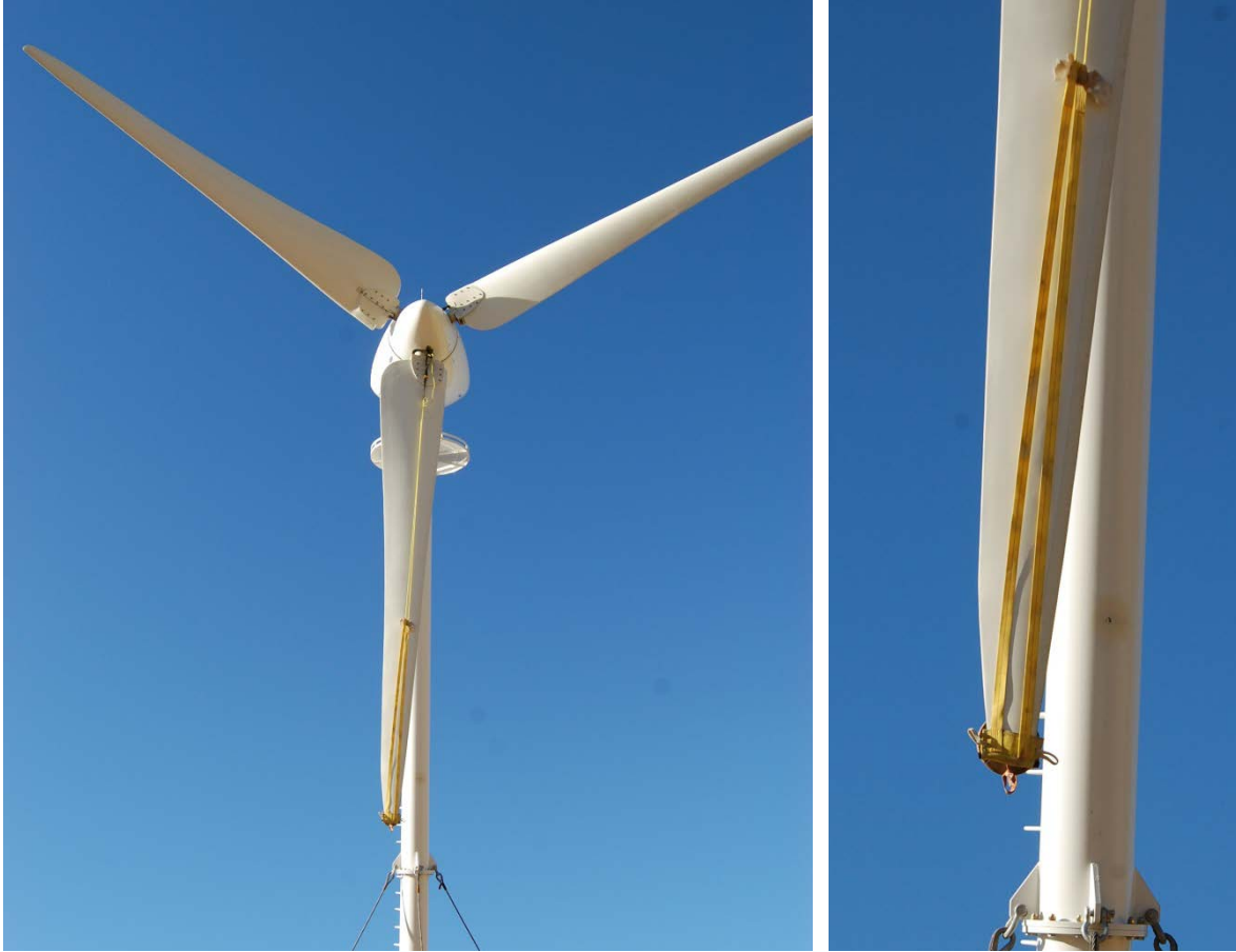
Figure 3. Rotor rotational inertia is measured using a weighted blade and measuring the frequency of oscillation. Photo courtesy of Windward Engineering
