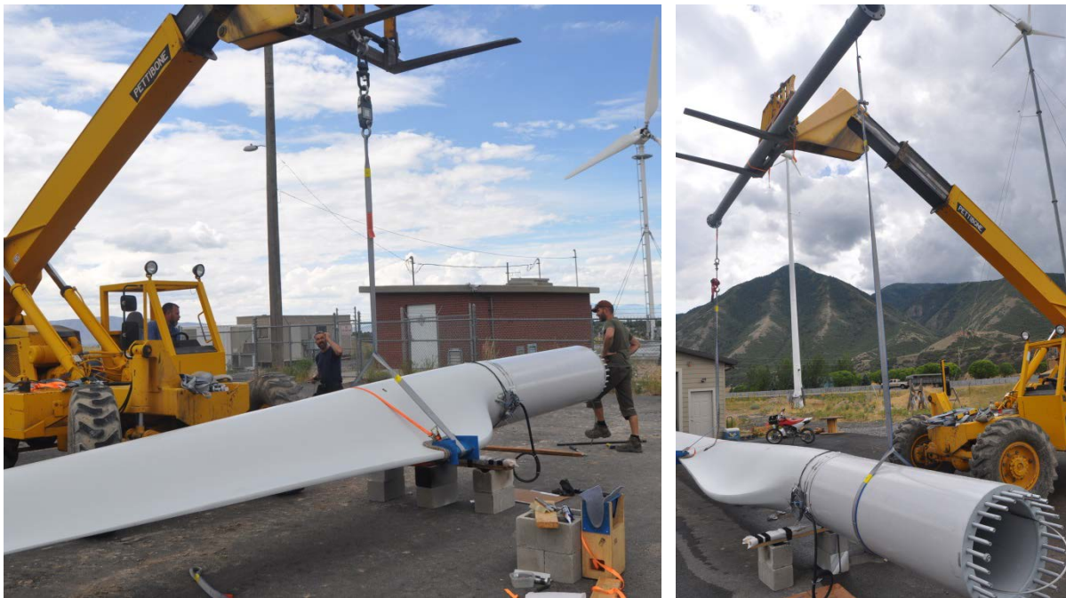
Figure 2. Measuring blade weight and center of gravity (left) and inertia with a bifilar pendulum (right). Photo courtesy of Windward Engineering
