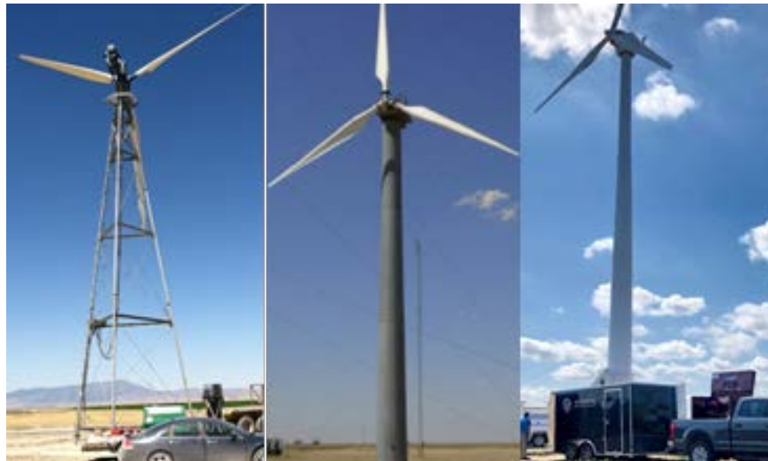
Figure 16. Three turbines with similar rotor-swept area but different rated power. Left: Kenetech 100 kW (227 m 2 ); Center: Micon 65 kW (200 m 2 ); Right: Eocycle 25 kW (196 m 2 ).
