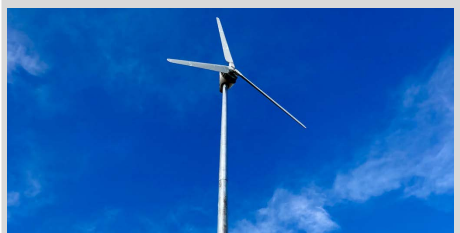
The QED PHX20, a three-bladed, 20-kW upwind turbine, is one of three modern wind turbines selected for installation at NREL's Flatirons Campus. The turbines will be used to conduct research focused on integrating wind energy in distributed applications. Photo from QED Wind Power
