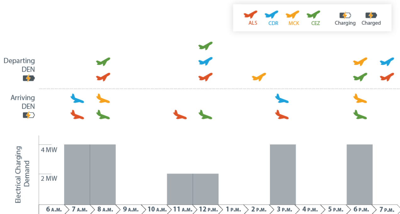
Figure 3. Potential load impacts of 2019 flight schedule between DEN and ALS, CDR, CEZ, and MCK
