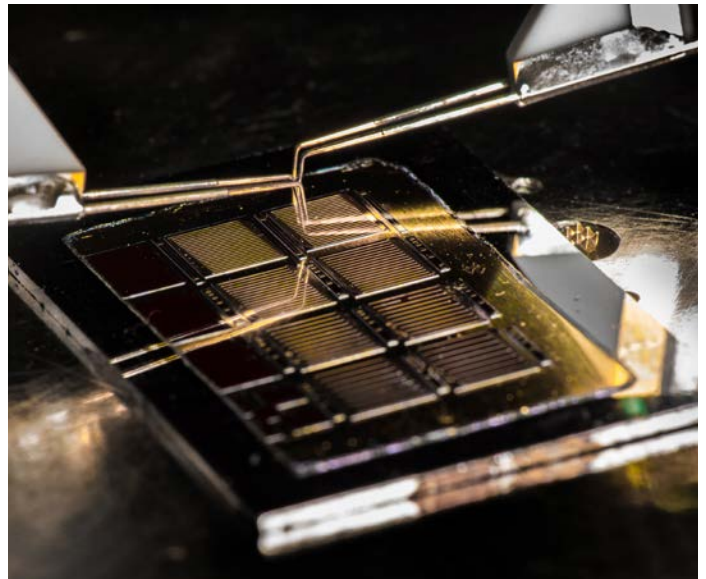
An NREL-developed metamorphic multijunction photovoltaic cell undergoing testing. Photo by Dennis Schroeder, NREL 32512
