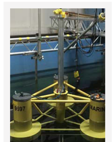
The validation campaign of the OC6-DeepC wind floating semisubmersible with rigid tower at the Maritime Research Institute of the Netherlands will help improve designs of semisubmersible turbine platforms. Photo by Amy Robertson, NREL
