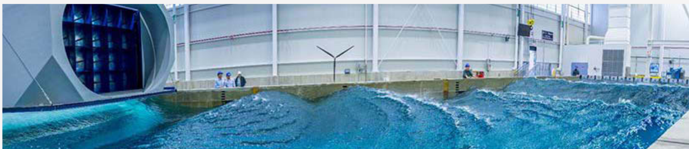
The W2 Ocean Engineering Laboratory at the University of Maine will be used to conduct combined wind and wave testing of wind turbines with advanced controls. Photo courtesy of the University of Maine
