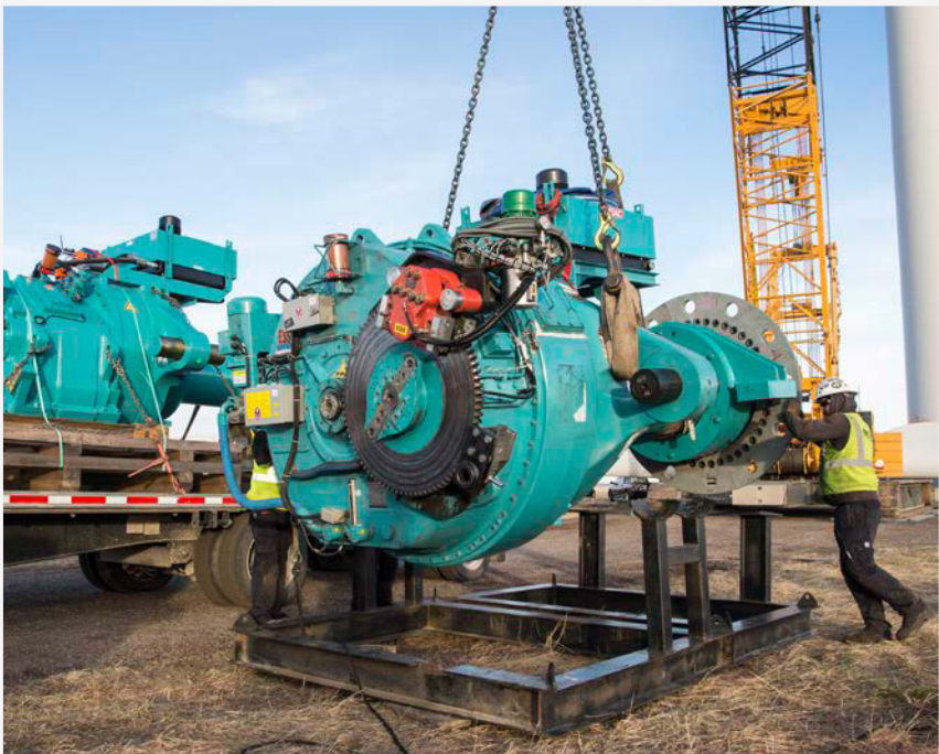
Resolving issues like bearing axial cracking and gear tooth micropitting increases drivetrain reliability, turbine availability, and reduces operation and maintenance costs. Photo by Dennis Schroeder, NREL 49408
