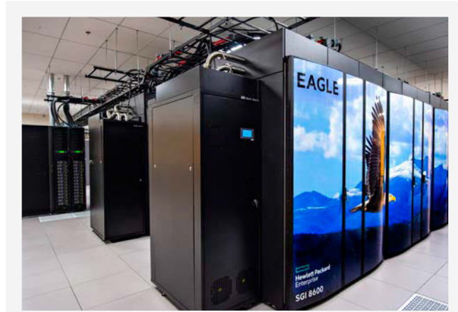
High-performance computing systems like Eagle will allow wind researchers to model wind resources in a manner that more accurately captures the myriad of calculations to grasp the underlying physics at play at wind power plants. Photo by Dennis Schroeder, NREL
