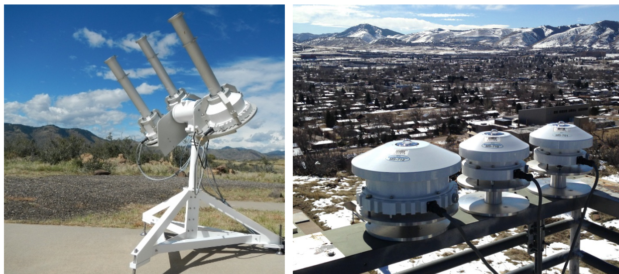
Figure 5-2. (Left) Three field spectroradiometers mounted on a solar tracker to sense the direct normal spectrum. Photo by NREL. (Right) The same three spectroradiometers but mounted horizontally to sense the global horizontal spectrum. Photo by Christian Gueymard
