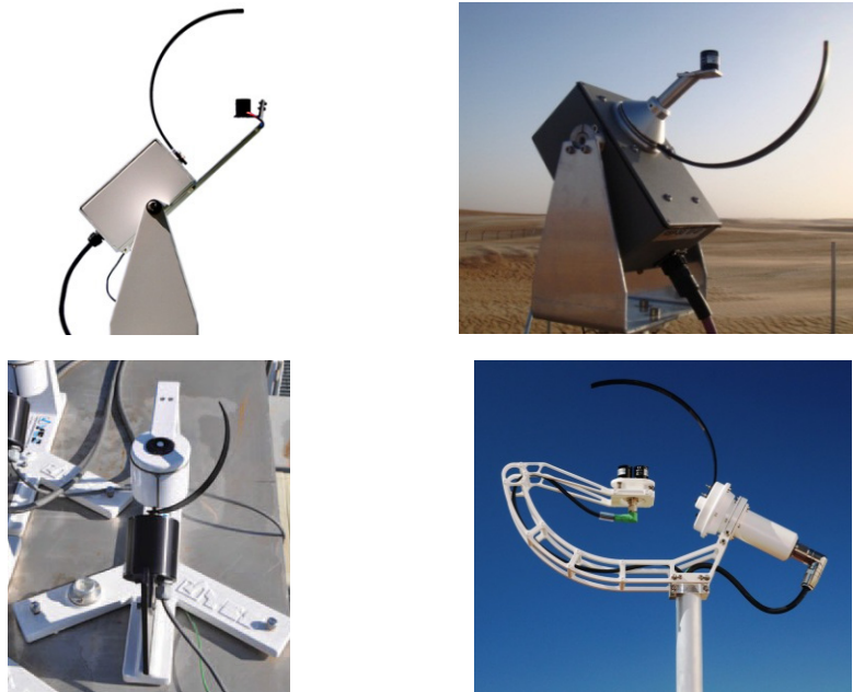
Figure 3-15. Four commercially available RSIs (clockwise from top left): Irradiance, Inc., model RSR2; Reichert GmbH RSP 4G; Yankee Environmental Systems, Inc., model SDR-1; and CSP-Services GmbH Twin-RSI. Photos by (clockwise from top left) Irradiance, Inc.; CSP-Services; NREL; and CSP-Services
