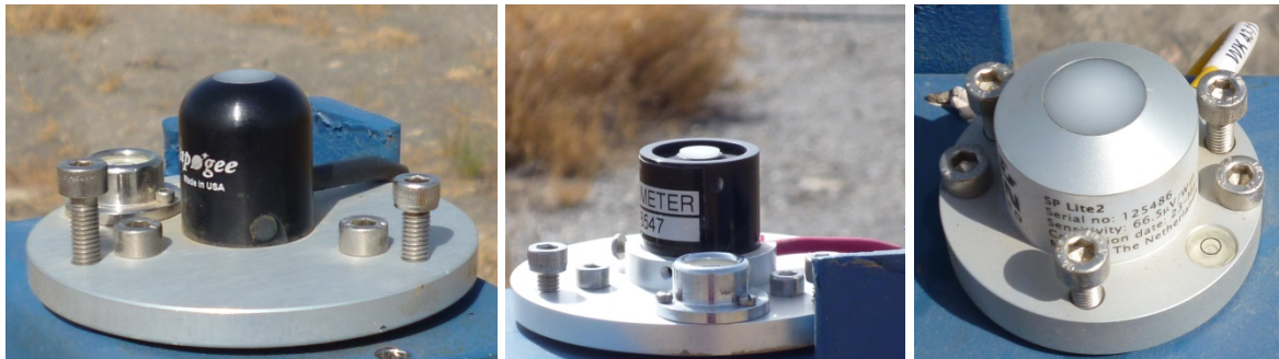
Figure 3-10. Selected photodiode sensors with different diffuser geometries. Photos by DLR
