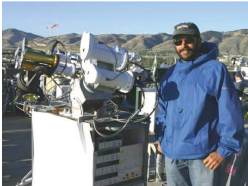
Figure 3-5. Multiple electrically self-calibrating absolute cavity radiometers mounted on solar trackers with control and data acquisition electronics. Photo by NREL
