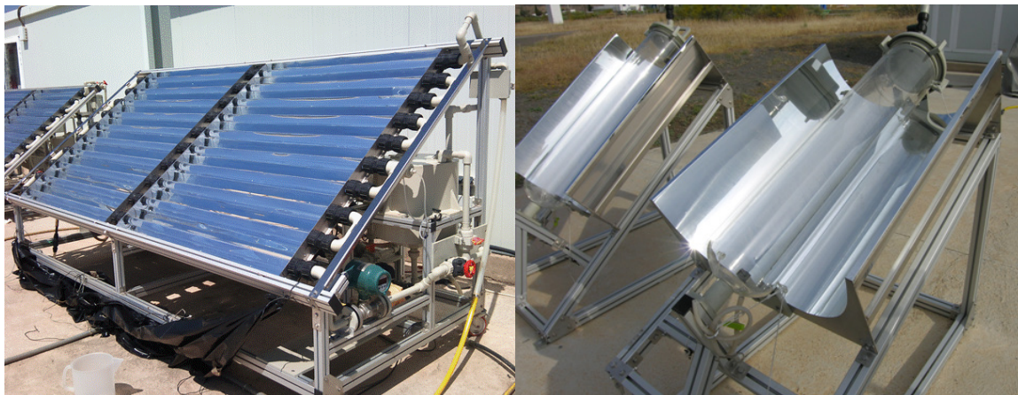
Figure 9-18. Compound parabolic collector photo reactors installed at Plataforma Solar de Almería for solar water disinfection applications: (left) compound parabolic collector-SODIS and (right) FITOSOL-2 . Photos from Plataforma Solar de Almería, CIEMAT
