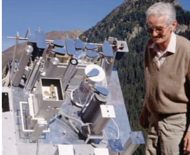
Figure 3-6. The World Standard Group of six absolute cavity radiometers is used to define the WRR or DNI measurement standard. Photo by NREL
