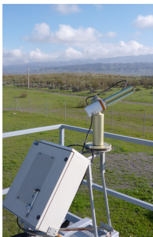
Figure 5-1. AERONET sun photometric station at CIEMAT's Plataforma Solar de Almería. Photo from DLR
