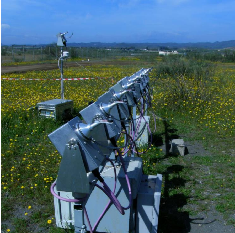
Figure 3-17. RSI calibration station at CIEMAT's Plataforma Solar de Almería. Photo by DLR
