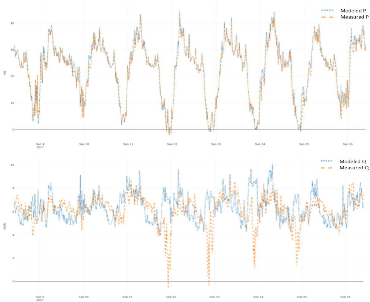
Figure 36. Measured versus modeled real (top) and reactive (bottom) power at the service transformer of the Cluster 1 secondary
