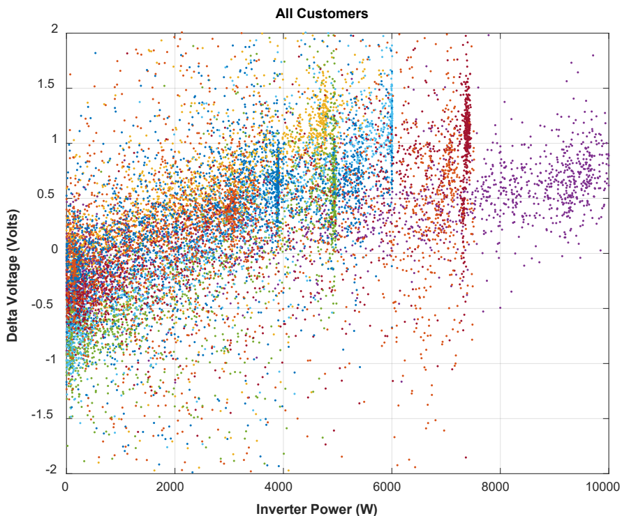
Figure 22. Behind-the-meter voltage rise for all string inverter customers as a function of inverter output power
