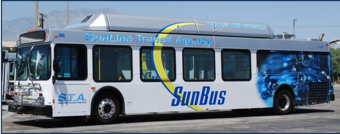
Figure 3. New Flyer CNG bus at SunLine
