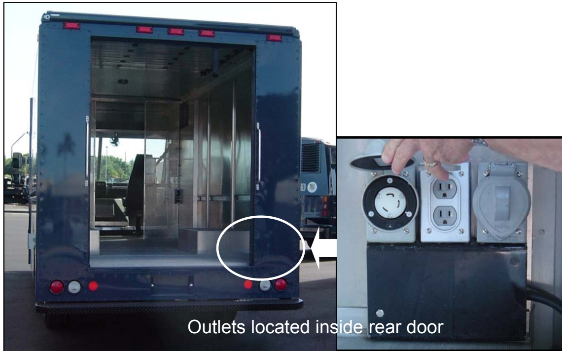
Figure 5. The fuel cell van is equipped with outlets to supply power in the field
