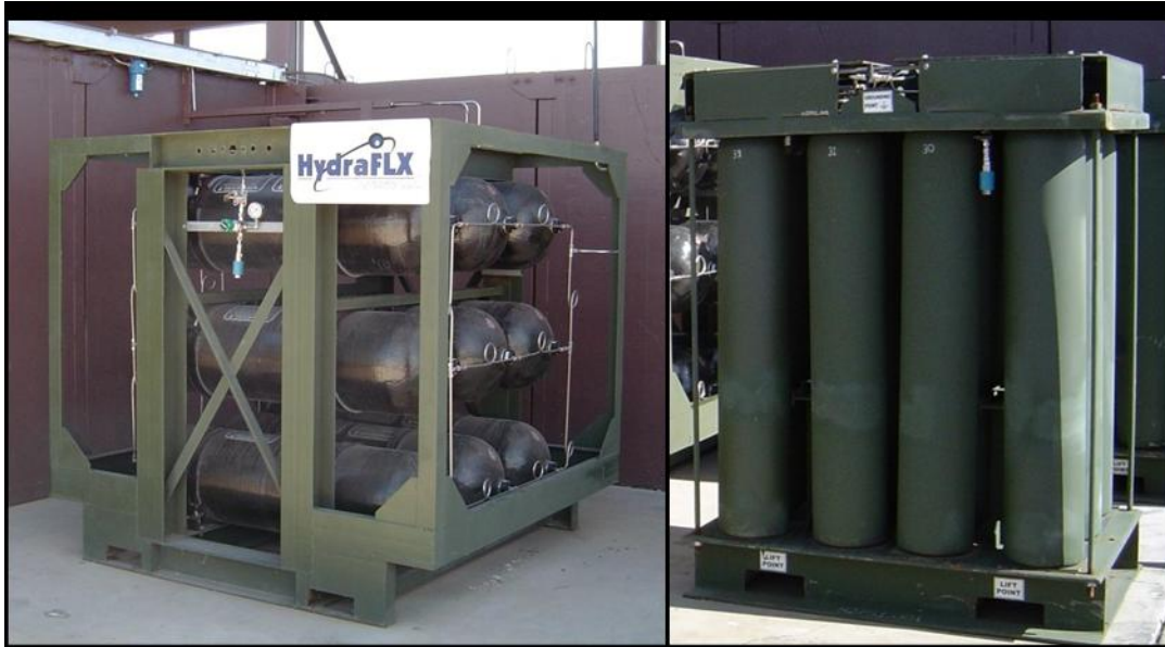
Figure 9. Primary hydrogen storage (left) and portable hydrogen lift pack (right)
