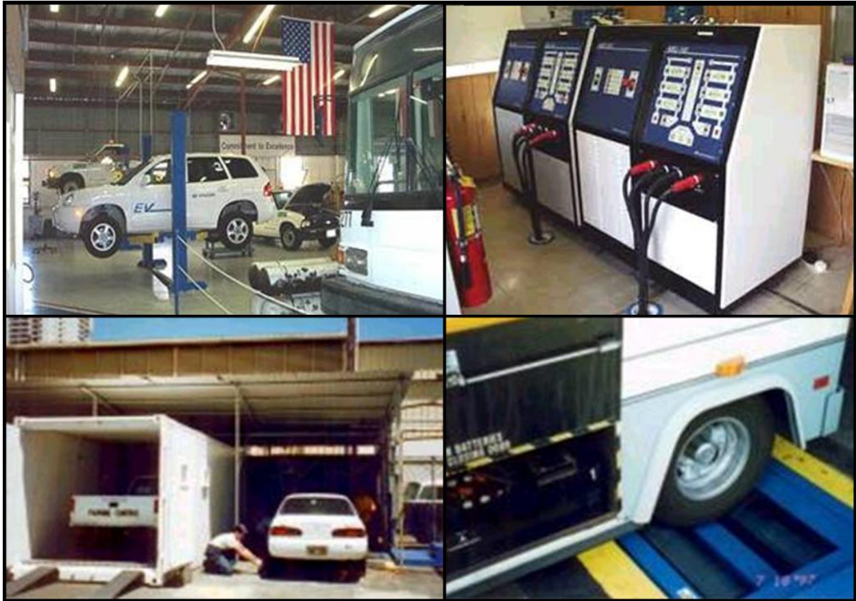
Figure 11. HCATT's facilities include vehicle lifts (top left), 2 ABC 150s (top right), an environmental chamber (bottom left), and a chassis dynamometer (bottom right).
