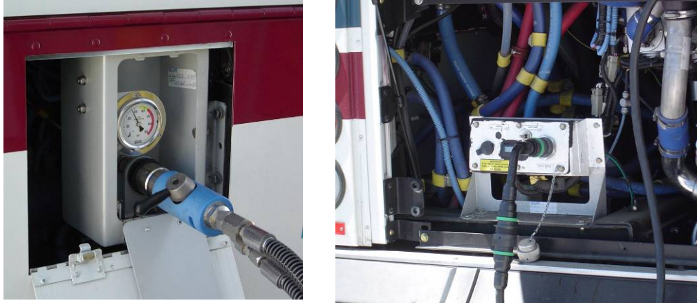
Figure 5. Hydrogen fueling connection (left) and communications connection (right) on the FCB
